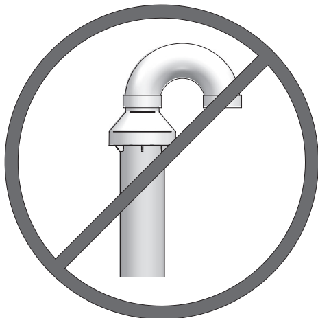
Figure 5-5 Do Not Install U-Bend to Rain Cap
